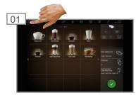
Switch to Maintenance level. Authenticate with the PIN code, if necessary. The factory-set PIN code is
